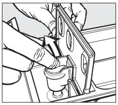
■ Remove the siphon from compartment ⊗ and rinse under warm running water.
